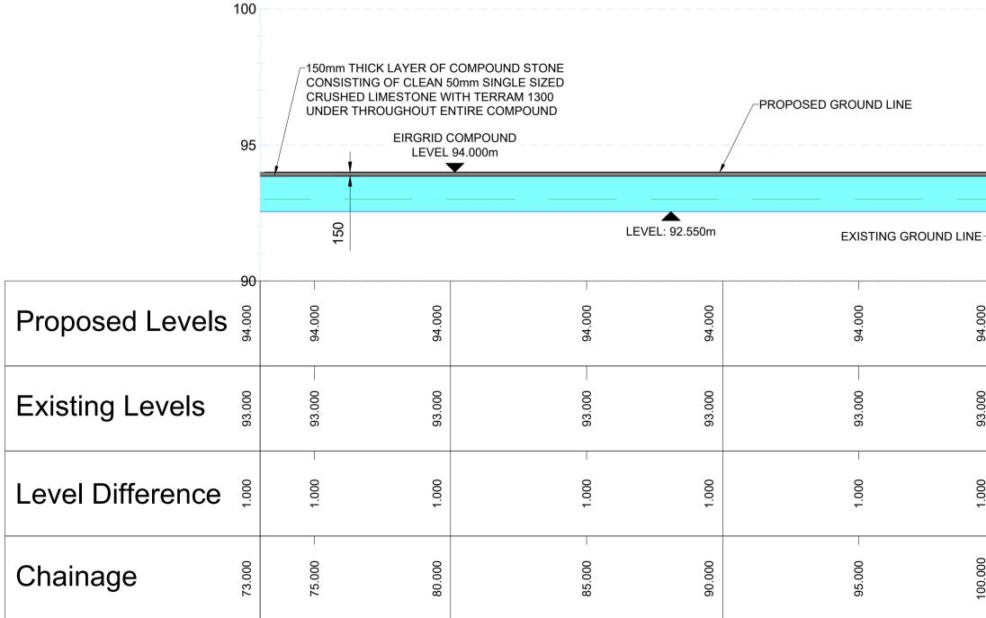
**SECTION A - PART 1** CH0.0M TO 73.0M SCALE H 1:125 , V 1:125
